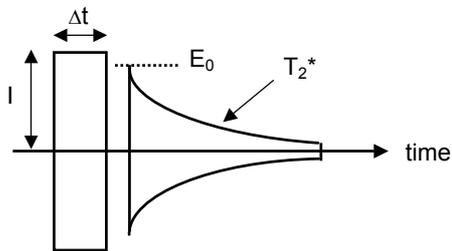
Figure 6. Envelopes of the excitation pulse and of the magnetic resonance relaxation signal:  $I$  is the intensity of the current,  $\Delta t$  its duration,  $E_0$  the initial amplitude of the signal,  $T_2^*$  its time constant
