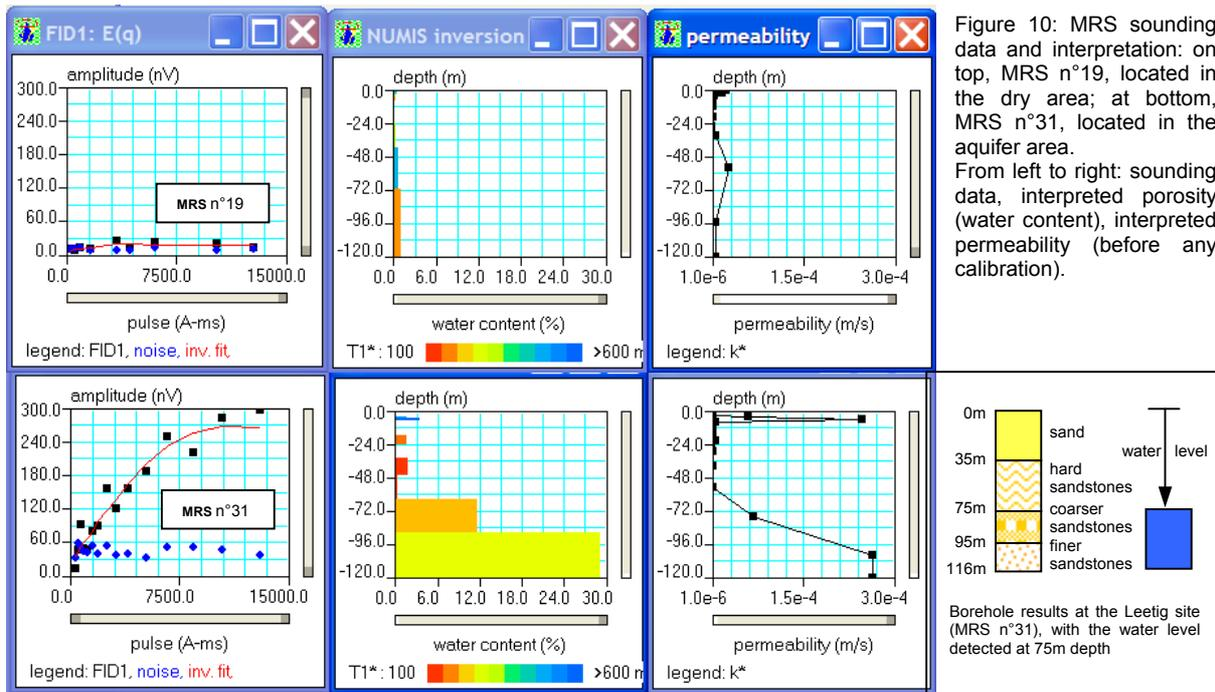
Figure 10: MRS sounding data and interpretation: on top, MRS n°19, located in the dry area; at bottom, MRS n°31, located in the aquifer area. From left to right: sounding data, interpreted porosity (water content), interpreted permeability (before any calibration).
