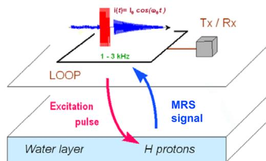
Figure 5: Principle of the magnetic resonance method
