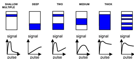
Figure 7: Typical magnetic resonance responses of aquifer layers, for various types of thicknesses and depths.
