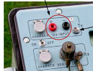
external transmitter battery plug
