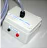
Rear side of the module with plugs for battery connection
