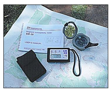
Four operating modes offer various methods of drift compensation, as well as a scan mode. Power is from two small lithium camera type batteries that will typically give 80 hours of operation. As the SM-30 features an automatic shut off after three minutes the batteries can be expected to last quite some time.
