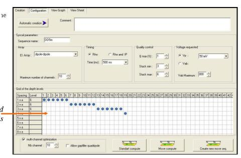
• Creation of the *Standard* sequence, or a *Move* sequence (defining the number of electrodes to be shifted) in case of long profiles acquisition.
